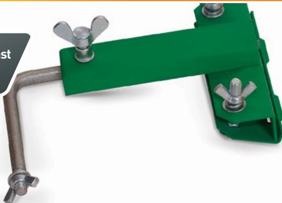
The adjustable bracket holds the blast gun at a specific position while you lift and manipulate the part under it. It helps reduce window frosting by keeping the blast pointed away from the glass. Adjustable gun bracket usually used in conjunction with a turntable.
