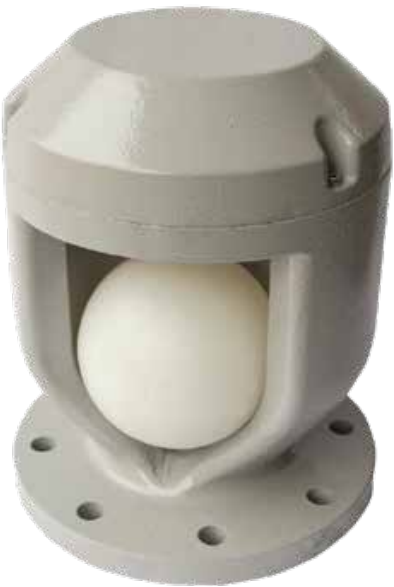
AIR VENT HEADS, DIN PN10/ PN16 FLANGED, BALL TYPE FCD450 BODY, STAINLESS STEEL TRIM - WITH CLASS TYPE APPROVAL CERTIFICATE HOT DIP GALVANIZED, SUITABLE FOR USE AT BOTH OIL & WATER TANKS.
