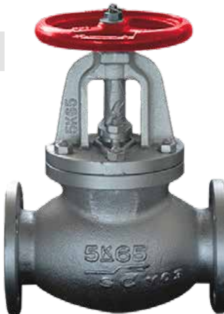
GLOBE VALVES, JIS 5K - WITH DNV-GL CLASS CERTIFICATE CAST STEEL BODY, STAINLESS STEEL TRIM, SCREW DOWN NON RETURN (SDNR)
